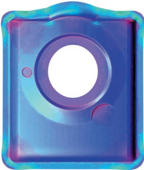
Simulation of the deep drawing process: washing machine front panel
